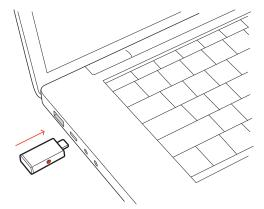
2 Connection is successful when you hear "PC connected" and the USB adapter turns solid. **NOTE** *Adapter design may vary.*
