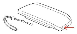
1 Insert the loop through one side of the slot and push through to the other side.
